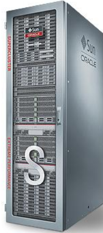
SuperCluster T5-8 2 * T5-8 compute nodes QDR (40 Gb/sec) InfiniBand
