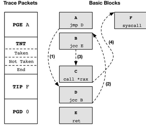
Figure 1: Following control flows using trace packets.
