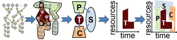
**Figure 1:** Steps taken by GRAPHENE from a DAG on the left to its schedule on the right. Troublesome tasks  $T$  (in red) are placed first. The remaining tasks (parents  $P$ , children  $C$  and siblings  $S$ ) are placed *on top* of  $T$  in a careful order to ensure compactness and respect dependencies.
