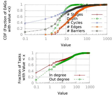
Figure 5: Characterizing structural properties of the DAGs
