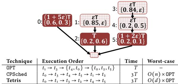
Figure 2: An example DAG where a packer (Tetris [37]) and a Critical Path scheduler take  $3 \times$  the optimal algo OPT. Here, GRAPHENE is close to OPT (see §2.2). Assume  $\varepsilon \rightarrow 0$ .
