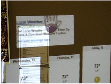
**Figure 7:** SURROUNDWEB maps natural gestures to mouse events. Here, the user uses a standard “push” gesture to tell SURROUNDWEB to inject a click event into the web application.
