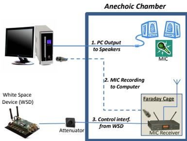
Figure 10: Anechoic chamber setup for audible interference tests.
