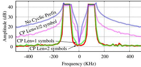
**Figure 16:** Strokes with varying CP in the frequency-domain.
