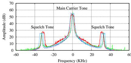
Figure 1: Spectrum signature of 6 idle mics.
