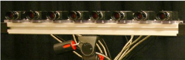
Figure 5. Our array of 8 VGA resolution video cameras.
