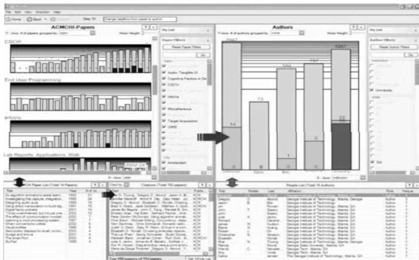
Figure 8. A screenshot of NetLens, an interactive system to explore networks using simple bar charts. Users filter different attributes of the network by clicking on corresponding bars. NetLens provide the textual result on the lower windows.
