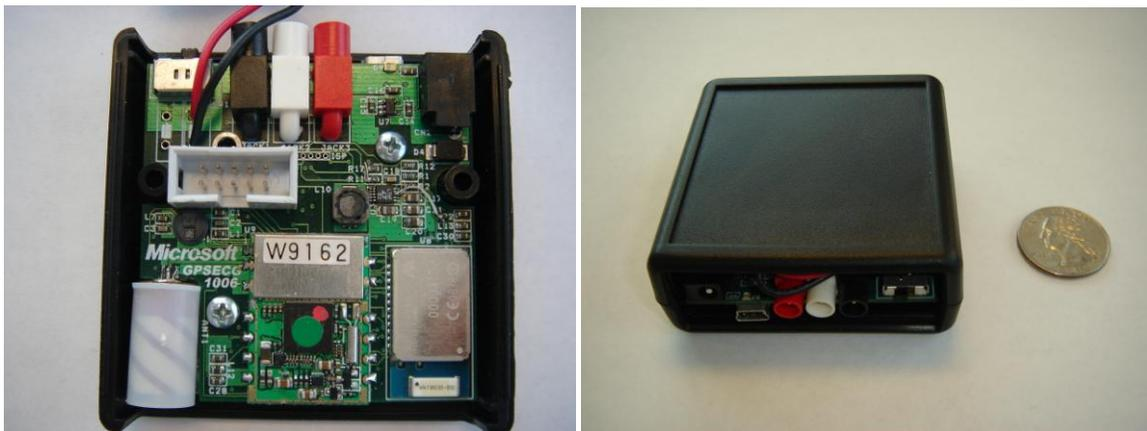
**Figure 1.** Prototype sensor board that includes GPS, accelerometer, pressure sensor, temperature, Bluetooth, and battery.
