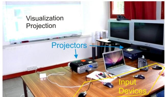
**Figure 1:** An example of a low-cost setup for co-located collaborative data analysis using four mice, two projectors, and a wall for projection.
