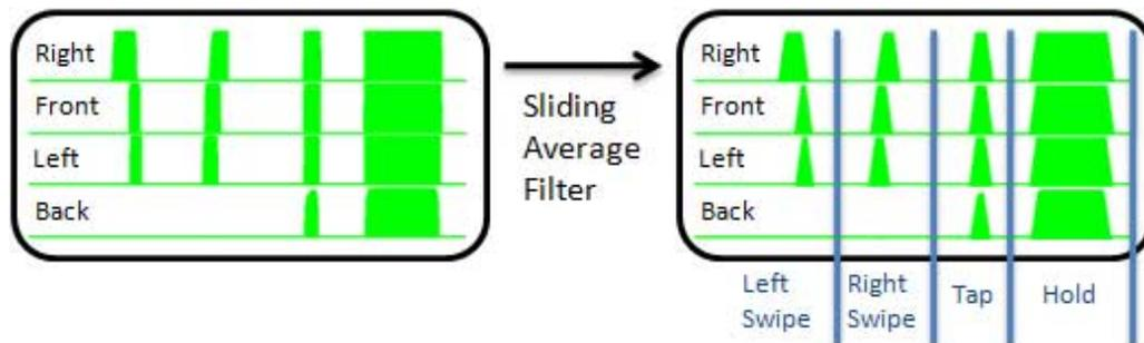
Figure 2. Example proximity sensor signal and processing. Each row represents the proximity data from a different sensor. The box at right shows the effect of a sliding average filter and examples of our four tongue gestures.
