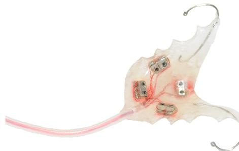
**Figure 1.** Our prototype optical tongue sensing retainer.
