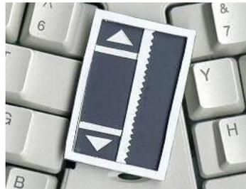
Fig. 13. Scrolling strip with absolute function in the "sawtooth" area on the right side of the strip.
