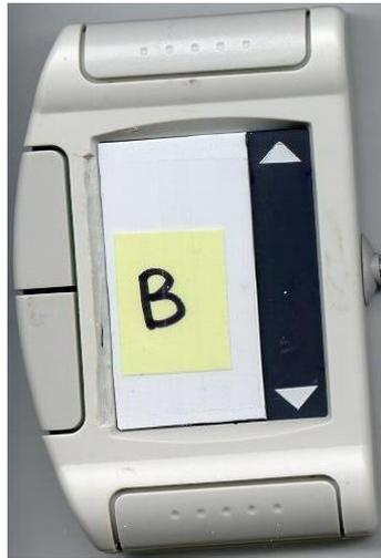
Fig. 4. Prototype B, a scrolling strip without arrow separations.
