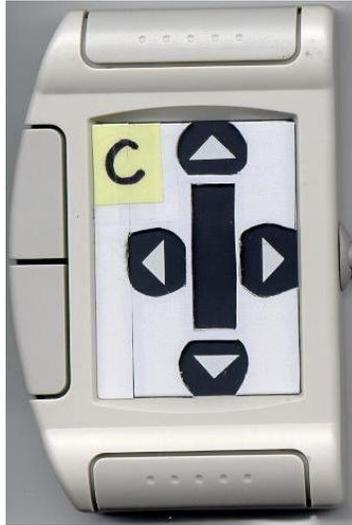
Fig. 6. Prototype C, a scrolling strip with horizontal arrows
