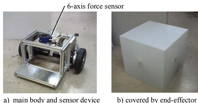
a) main body and sensor device      b) covered by end-effector
