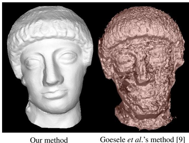
Figure 5. Comparison with a multi-view stereo method without a photometric constraint [9] using the statue scene. 93 images are used as input for both methods.
