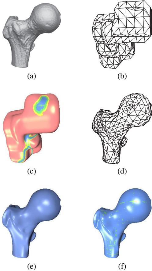
**Figure 8. Ball joint: (a) Unorganized point data. (b) Initial mesh. (c) Initial error. (d) Optimized mesh. (e) Subdivision surface. (f) Final error. No. of data points: 137062. No. of control points in the optimized mesh: 489.**
