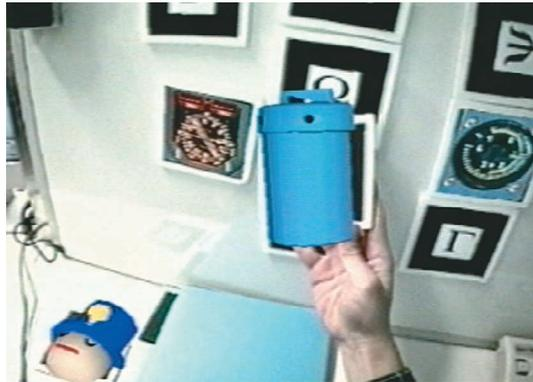
**Figure 5. Copying data from the clipboard to an empty data tile.** The user moves the tile close to the virtual clipboard and, after a one-second delay, the virtual instrument slides smoothly onto the data tile.
