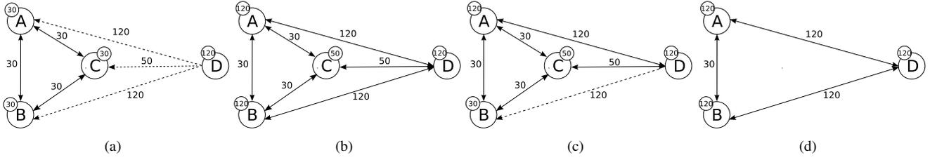
**Figure 1. Operation of the topology control algorithm: a simple example ( $K = 2$ ). Values on edges represent distances while the number on each node shows the node’s transmission range.**
