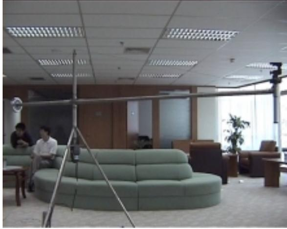
Figure 1: Capturing device of concentric mosaics.
