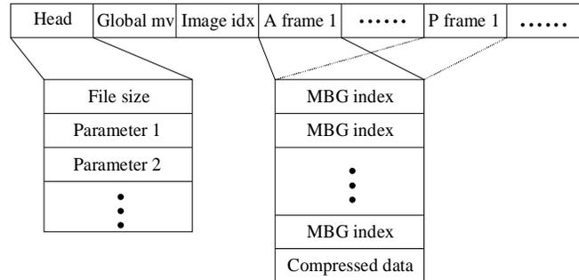
Figure 5: Syntax of the compressed concentric mosaics file.
