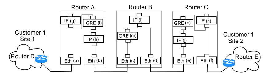
One possible path (using GRE-IP Tunnel) a, g, l, h, b, c, i, d, e, j, n, k, f
