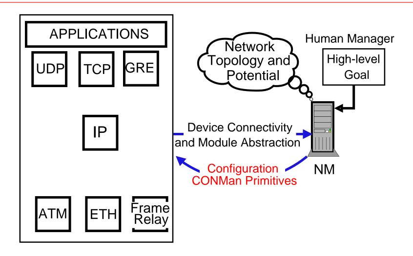
NM uses CONMan primitives to manipulate abstraction elements and configure network devices
