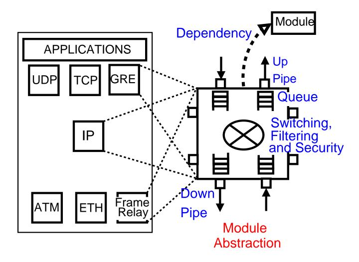
Module Abstraction: Mgmt Interface of a module Applies to (almost) all data-plane protocols
