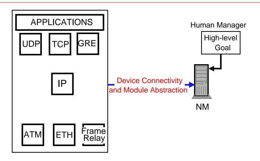
Each device's connectivity and the abstraction for its modules are sent to the NM
