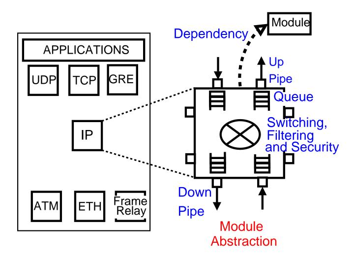
Module Abstraction: Mgmt Interface of a module Models the protocol's potential and dependencies
