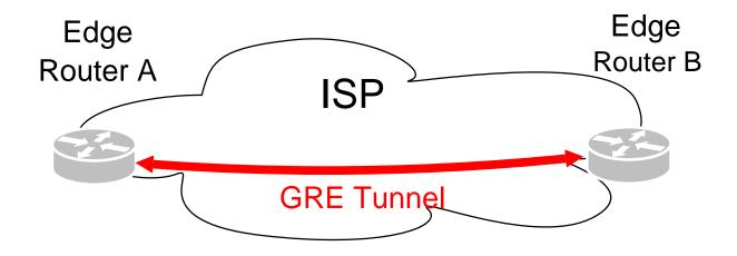
A GRE tunnel between edge routers A and B
