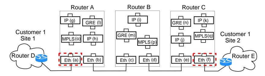
**High-level goal**: Configure connectivity between the customer-facing interfaces < ETH,A,a> and < ETH,C,f> for traffic between C1-S1 and C1-S2
