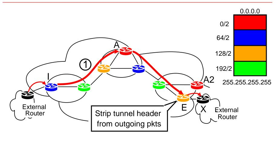
Egress Router strips the tunnel header off outgoing packets
