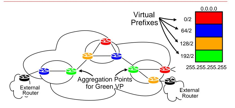
Assign Virtual Prefixes to the routers Routers only have routes to a fraction of the address space
