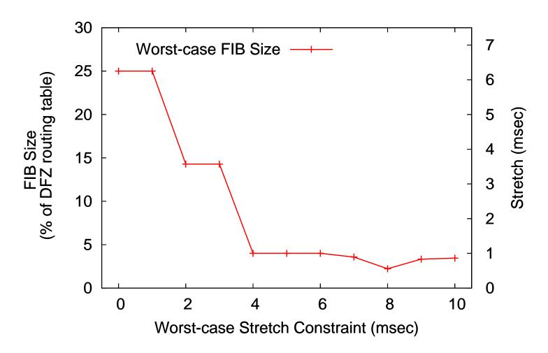
FIB Size reduces as Stretch constraint is relaxed
