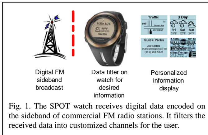
Fig. 1. The SPOT watch receives digital data encoded on the sideband of commercial FM radio stations. It filters the received data into customized channels for the user.
