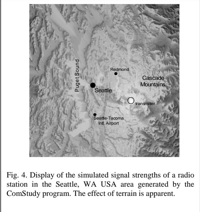
Fig. 4. Display of the simulated signal strengths of a radio station in the Seattle, WA USA area generated by the ComStudy program. The effect of terrain is apparent.
