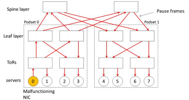
Figure 5: The PFC pause frame storm caused by the malfunctioning NIC of one single server (server 0).
