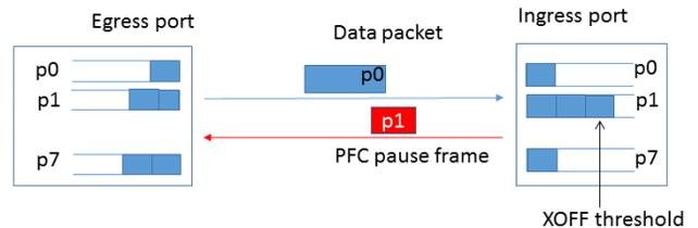
Figure 2: How PFC works.
