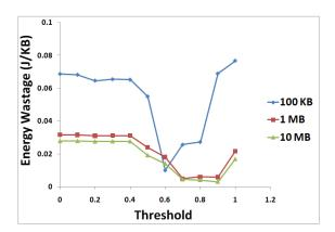
Figure 10: Expected Energy Wastage per KB for different file transfers
