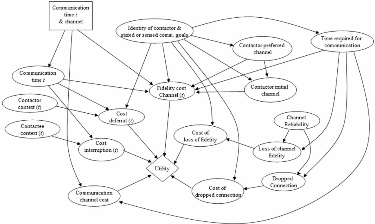
Figure 1. Decision model for best-means communication actions, represented as an influence diagram. Utility maximization algorithms identify the communication action with maximum expected utility given the expected cost of interruption, the cost of communication deferral, the cost of channel usage, and the losses in fidelity associated with the use of alternate modalities.
