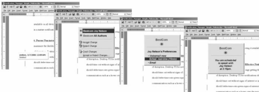
Figure 10. Bestcom service as embedded in MS Word. Here, best-means communication is invoked via a menu item. In this case, the Bestcom server reports back a list of recommended communications actions, sorted by the contactee’s preferences.
