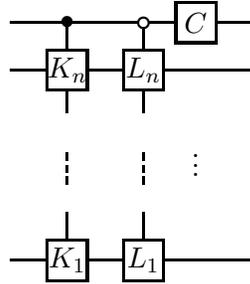
**Figure 8:** Quantumcircuit for the diagonal matrix  $D_1$ .
