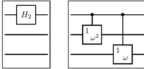
**Figure 3:** For length  $N=8$ , only three qubits are necessary. The circuit on the left implements  $(F_2 \otimes \mathbf{1}_{N/2})$  and the other realizes the twiddle matrix  $\mathbf{1}_4 \oplus \text{diag}(1, \omega, \omega^2, \omega^3)$ .
