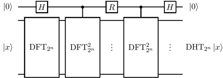
**Figure 10:** Circuit realising a quantum Hartley transform
