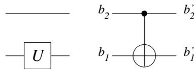
**Figure 1:** The Feynman notation for the single qubit gate ( $\mathbf{1}_2 \otimes U$ ) and for a controlled NOT operation  $|b_2' b_1'\rangle = |b_2 b_2 \oplus b_1\rangle$ .
