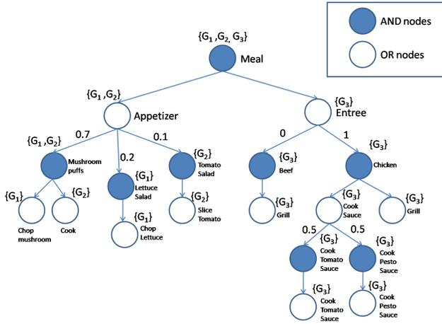
**Figure 1: A Probabilistic recipe tree for the meal preparation example. Each node is associated with an action (e.g., make mushroom puffs), and a set of agents to perform the action (e.g.,  $\{G_1, G_2\}$ ).**
