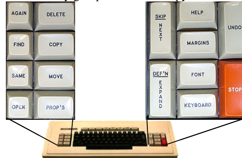
Figure 2: The Xerox Star keyboard (circa 1981) with detail of the function key groups. Note that Copy is on the left.
