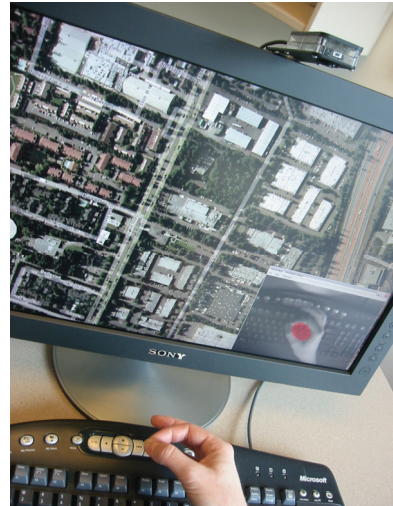
Figure 1: TAFFI prototype includes a USB camera mounted on the top of the display, looking at the user's hand above the keyboard. Here TAFFI is used to navigate Virtual Earth aerial imagery.
