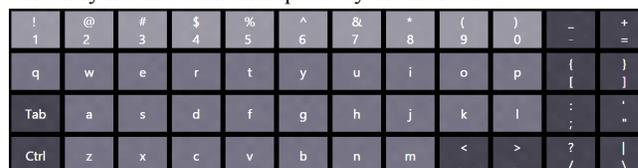
Fig. 1 The stroke-augmented graphical QWERTY keyboard tested in our studies. Note that the keyboard looks familiar despite the absence of the *Space*, *Backspace*, *Shift*, and *Enter* keys.
