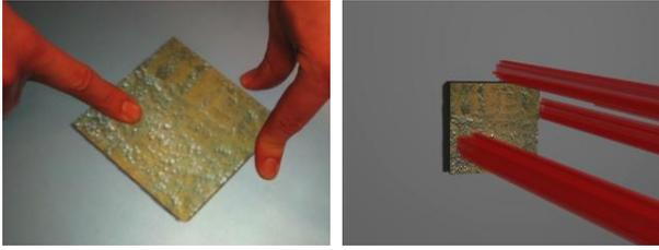
**Figure 2. Particle proxies approximate the shape of multiple contacts. Left: applying friction from the top, and collision from the side to grip a block. Middle: long proxy particle objects (red) illustrated.**
