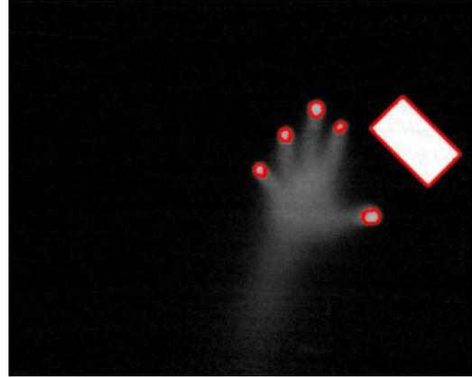
**Figure 3. Example image from diffuse-illumination table showing fingertips in contact and business card (face up) on the table. Extracted contours are in red.**
