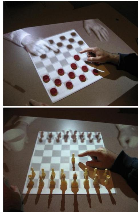
**Figure 1. Playing checkers and chess with a remote player using PlayTogether. The remote player's game pieces and hands are projected, superimposed on the local player's real board and pieces. In both cases, hands and pieces on the far side of the table are projected. Hands and pieces on the near side, and game board, are real.**
