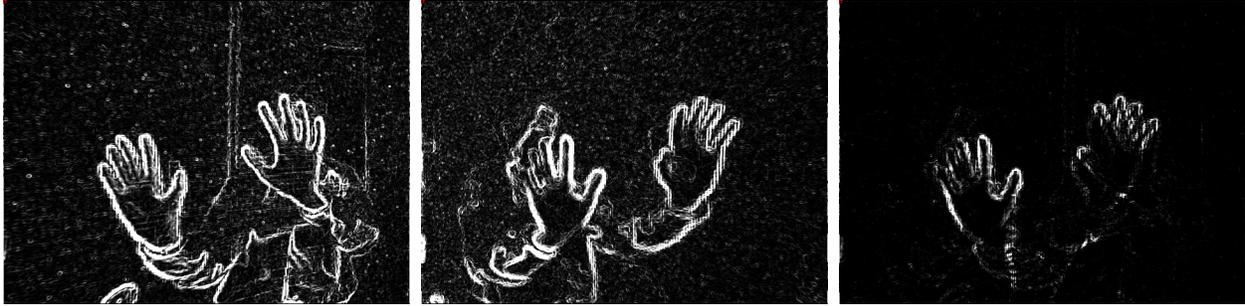
**Figure 5** Example of TouchLight image processing. Edge images from both cameras (left and middle) are combined to produce a touch image (right). In this case the hand on the left is flat on the display surface, while only the fingertips of the hand on the right are touching the surface.
