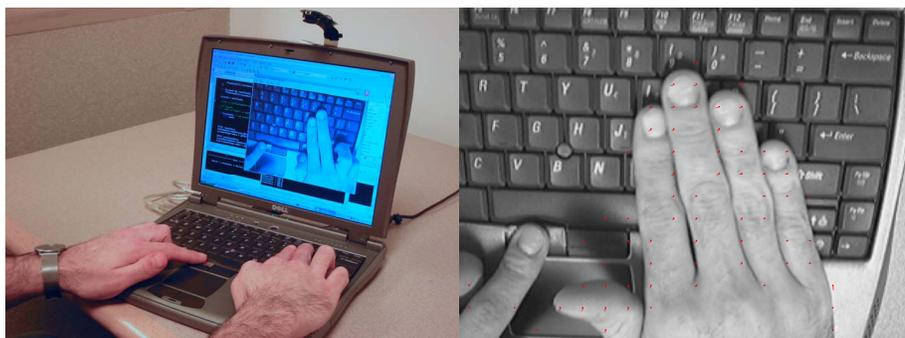
**Figure 1** Left: FlowMouse prototype with screen-mounted camera facing down on keyboard and user's hands, and touch sensitive strip on left mouse button. Right: Example image capture from camera.
