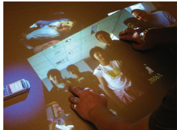
Figure 8. Photos may be scaled, rotated and moved on the desk by using one or both hands. Optical flow techniques are used to recover the motion of the hands. This motion is then modeled as a combination of simultaneous rotation, scaling and translation movements. An individual photo is brought to the top of the stack of multiple photos by touching any part of the photo with an outstretched finger.
