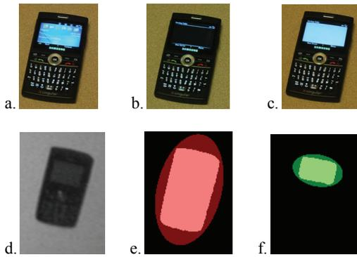
Figure 6. Visible light modulation. Samsung SGH-i607 smartphone (a) is not equipped with an IRDA port so BlueTable modulates onscreen graphics instead. Pulses are generated by changing the onscreen graphics from black (“on” pulse) (b) to white (c). The device is initially detected from the IR signal as before (d and e), but the pulse is detected in the visible spectrum using a second camera (f).
