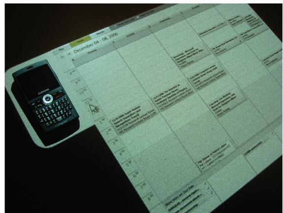
Figure 10. Mockup of a complex user interface (calendar application) that spills out of a mobile device onto BlueTable.
