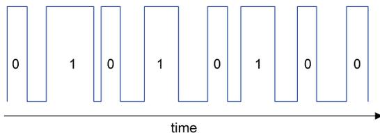
Figure 5. Pulse width modulation, least significant bit first, for the 8 bit value 42, using direct control of IRDA port. Timings were collected on the host interactive surface system, from image analysis. Limits on the control of timing and sampling error contribute to inaccuracies in pulse width.
