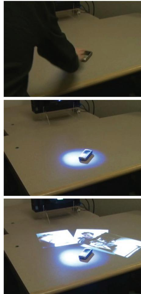
Figure 7. BlueTable prototype connects automatically to cameraphone via Bluetooth, transfers photos, and spills them onto interactive surface.
