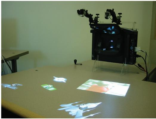
Figure 1. PlayAnywhere projection-vision interactive surface system uses a single camera, infrared illuminant, and a short-throw projector on a regular table surface.
