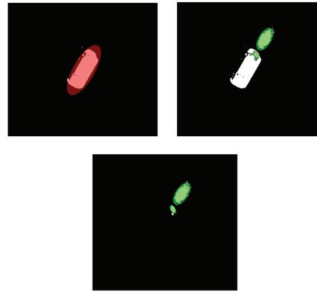
Figure 3. IRDA port blinking. Top left: phone shape detected, with fit ellipsoid model (red). Top right: infrared light detected at IR port and on surface (green). Bottom: infrared light is detected apart from phone shape by image differencing.
