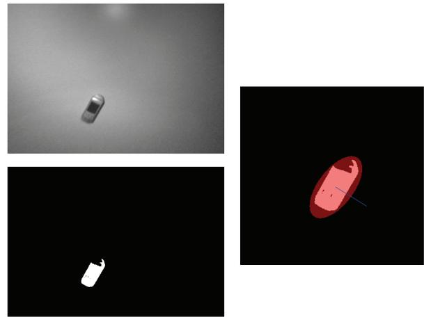
Figure 2. Upper left: input image with phone; Lower left: binarized image; Right: binarized image with ellipse fit (red).
