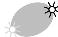
Figure 4. 180 degree ambiguity of ellipsoidal model is removed by determining at which end of the ellipse the infrared signal appears.
