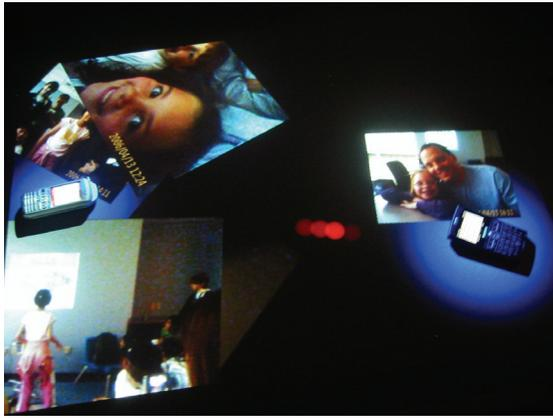
Figure 9. Support of multiple devices and transferring documents. Photos taken with the left cameraphone may be transferred via Bluetooth to the phone on the right by dragging photos onto its blue halo. The transfer is depicted visually by an animation (red) from the source phone to target phone.
