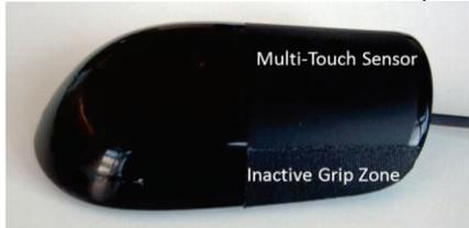
Figure 2. The Cap Mouse prototype (developed by [24]) used in our investigation: the labels mark the curved capacitive multi-touch sensor area and the inactive grip zone that can be used for gripping the mouse without touching the sensor.
