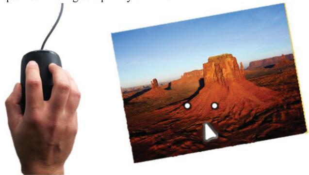
Figure 1. The multi-touch mouse device in use and the corresponding cursor and the touch points in the interface.
