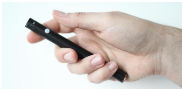
Figure 14: Custom IR laser pointer.
