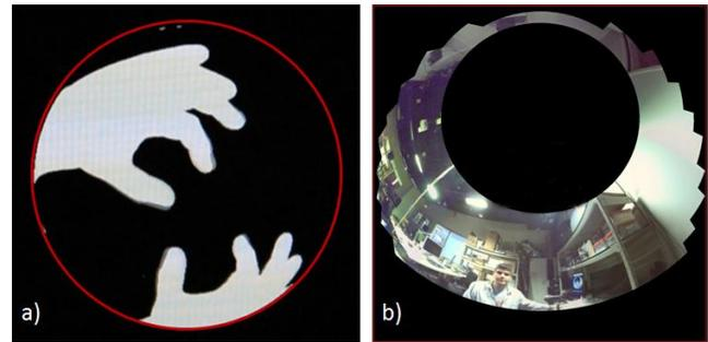
Figure 9: This image shows the distortions present when sensing and projecting in the dome: a) the binary camera image showing user's hands above the projector, and b) the pre-distorted image supplied to our projector which is necessary for correct projection in the dome for the 360 degree video conferencing application. Since our dome is a *tilted dome*, our visualization is uneven in order to appear horizontal in the dome, as seen in Figure 1a.
