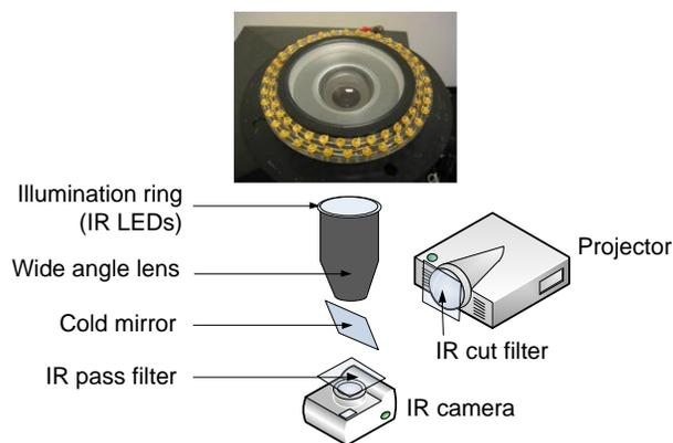
Figure 7. Schematic drawing of our omni-directional projector-camera unit. The detail image shows the wide-angle lens and the IR illumination ring.
