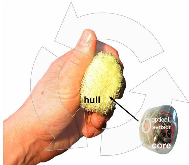
Figure 1: The core of soap is an optical sensor. The core can rotate freely inside soap's elastic hull. While pointing, users cause soap's core to rotate by applying off-axis pressure. The relative motion between core and hull is picked up by the optical sensor inside the core.
