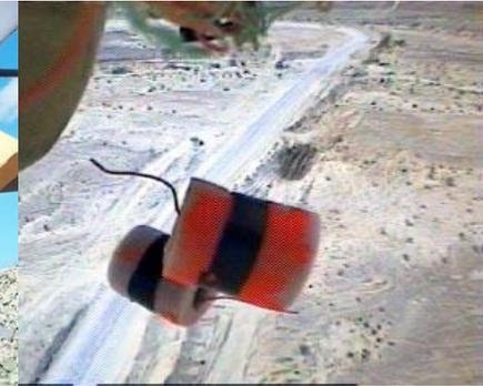
**Motes dropped from UAV, detect vehicles, log and report direction and velocity**
