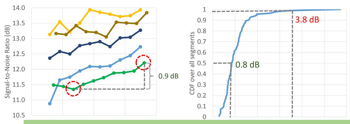
Different wavelengths need different modulation formats even though the path is shared
