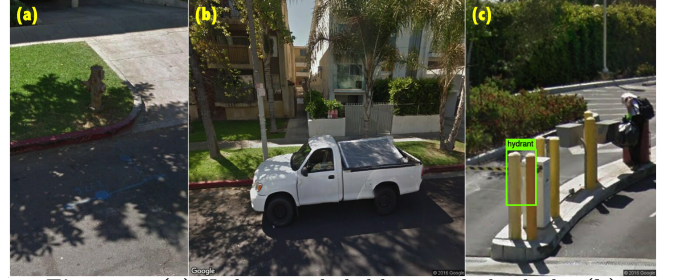
Figure 8: (a) Hydrant occluded by a parked vehicle. (b) Detection failure because hydrant is under the shade of a tree. (c) False positive detection of bollard as hydrant.
