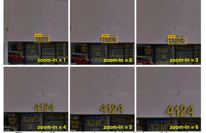
Figure 3: How zooming-in can help eliminate false positives
