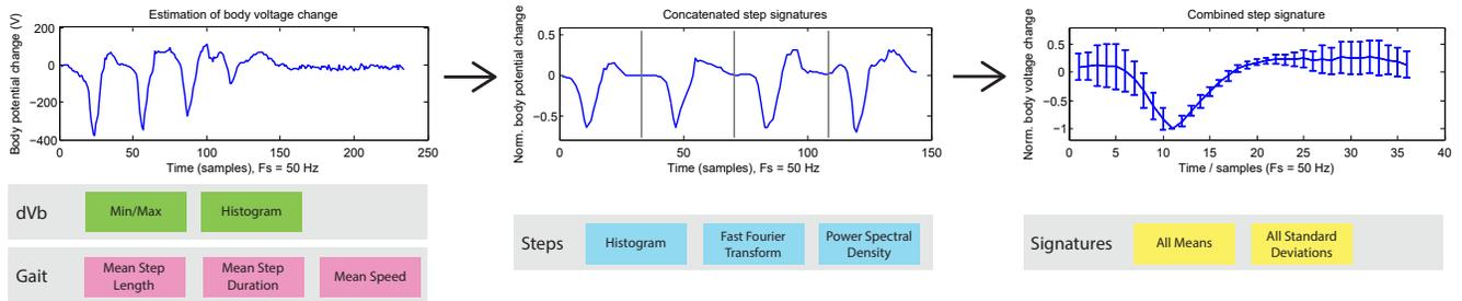
Figure 5: The feature extraction process for identification results in four feature sets: (1)  $dVb$  body electric potential, (2) *gait*-related, (3) a sequence of normalized *steps*, and (4) the combined and normalized step *signatures*.
