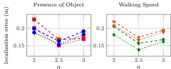
Figure 7: Interactions of  $\alpha$  values on median localization error plots with object (left, square data points indicate object present, circles no object present) and walking speed (right, triangles indicate normal speed, diamonds slow speed). Calibration level is marked with dotted lines (standard) and dashed lines (individual).
