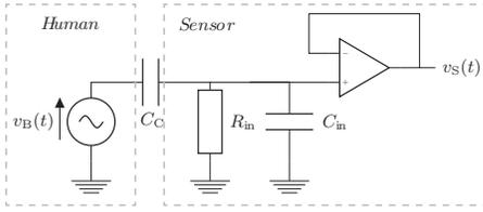
Figure 4: Electric potential sensor represented by an equivalent circuit (adapted from [13]).  $v_b$  represents the changing body electric potential, whereas  $C_C$  is the coupling capacitance which changes with the body-to-sensor distance.
