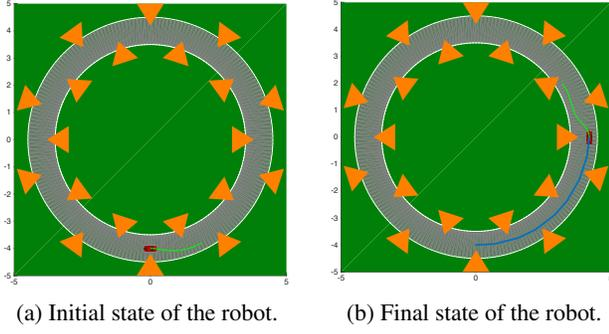
Figure 1: Autonomous robot reaching a final goal while avoiding obstacles. Here, the red car on the road shows the autonomous robot. The robot’s goal is to travel on the circular road while avoiding obstacles and staying within boundaries. The orange triangles represent the obstacles on the road. The green line on both figures shows the computed future trajectory of the robot for the next horizon. The blue line in 1b shows the trajectory computed and taken by the robot to reach its goal.
