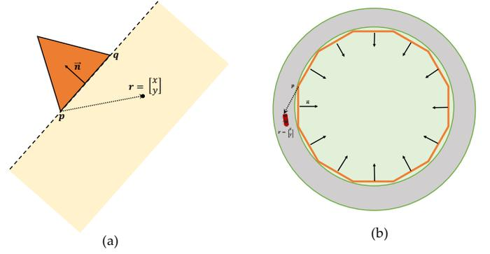
Figure 2: Obstacle avoidance by staying on one side of a hyperplane.  $\mathbf{p}$  and  $\mathbf{q}$  are the corners of an obstacle. We calculate  $\vec{\mathbf{n}}$  as the unit normal to this hyperplane. For a state with coordinates  $\mathbf{r}$  to be in the yellow region, the dot product of  $\vec{\mathbf{n}}$  and vector  $\mathbf{pr}$  must be negative. In (b), we show fitting a polygon to the inner circle in order to enforce staying out of the inner road boundary.
