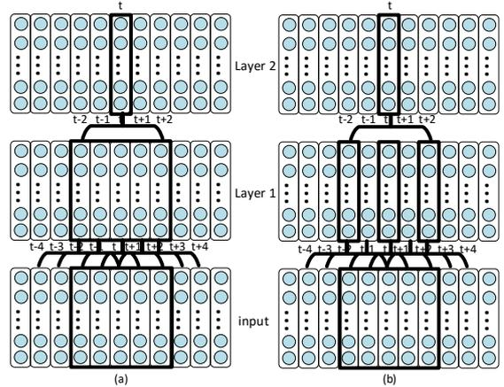
Figure 1: Illustration of the layer-wise context expansion.
