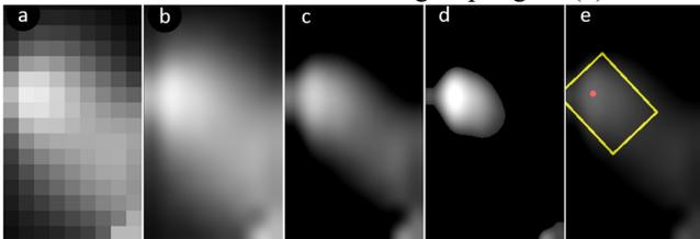
Figure 4. Image processing pipeline for fingertip extraction.
