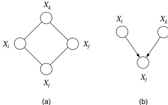
Figure 5: (a) An undirected graph in which  $X_i$  is independent of  $X_j$  given  $X_k$  and  $X_l$ , and  $X_k$  is independent of  $X_l$  given  $X_i$  and  $X_j$ . (b) A directed graph in which  $X_i$  and  $X_k$  are marginally independent but are conditionally dependent given  $X_j$ .
