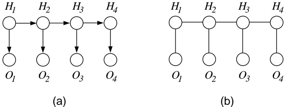
Figure 6: (a) A directed graph representation of an HMM. Each horizontal link is associated with the transition matrix  $A$ , and each vertical link is associated with the emission matrix  $B$ . (b) An HMM as a Boltzmann machine. The parameters on the horizontal links are logarithms of the entries of the  $A$  matrix, and the parameters on the vertical links are logarithms of the entries of the  $B$  matrix. The two representations yield the same joint probability distribution.
