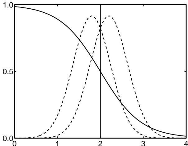
Figure 2: This shows the Gaussian class-conditional densities  $p(x|\mathcal{C}_1)$  (dashed curves) for a two-class problem in one dimension, together with the corresponding posterior probability  $p(\mathcal{C}_1|x)$  (solid curve) which takes the form of a logistic sigmoid. The vertical line shows the decision boundary for  $y = 0.5$  which coincides with the point at which the two density curves cross.
