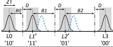
**Figure 5.** Cell configured with biased levels. The goal is to reduce drift-induced errors by equalizing the error rate of each individual level.
