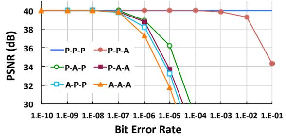
**Figure 7.** Image quality degradation with approximate bit streams. P denotes precise substrate, A denotes approximate substrate with BERs varying along the x-axis. The first letter represents control bits, the second represents run length bits, and the third represents refinement bits.
