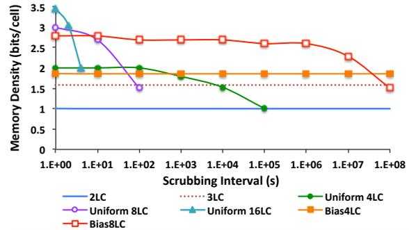
**Figure 10.** Density comparison (target UBER =  $10^{-16}$ ).
