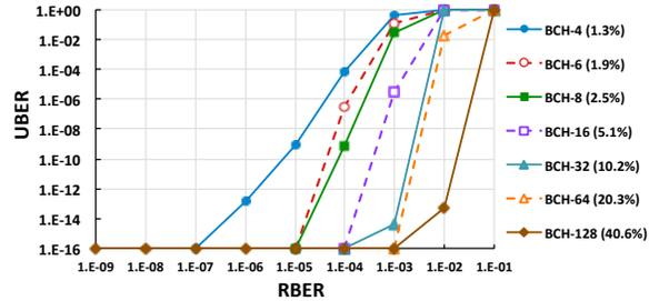
**Figure 13.** Capabilities and overheads of error correcting codes commonly used with Flash. Each code is able to correct the denoted number of errors in a 512-byte Flash sector and the associated ECC checker bits.
