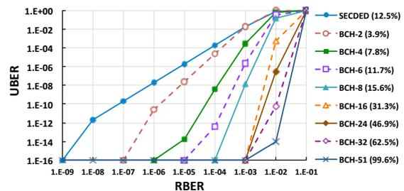
**Figure 11.** Capabilities and overheads of ECC (at 512 data bit blocks). SECDED corrects one error and detects up to two errors in 72 bits; each of the BCH codes corrects up to the denoted number of errors in 512 data bits plus overhead.
