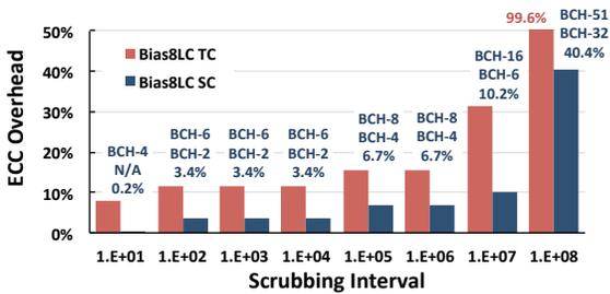
**Figure 12.** Trade-off between ECC storage overhead and scrubbing interval. Above each set of bars, the code in the first row is applied to all the bits in thorough correction (TC); the selective correction (SC) uses the first-row ECC for the control and run-length bits in MB1, and the second-row ECC for the control and run-length bits in other MBs, and leaves all refinement bits unprotected. The third row shows the total overhead.
