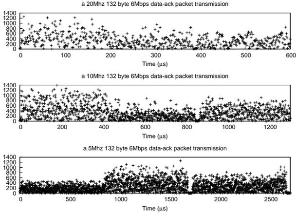
**Figure 5: A time-domain view of Data-ACK frames sent at 6Mbps OFDM at different widths. The Y-axis is  $\sqrt{I^2 + Q^2}$  for every sample.**
