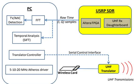
Figure 4: Functional block diagram of the KNOWS platform.
