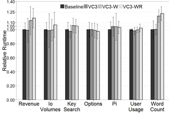
**Fig. 5:** Execution time of running MapReduce jobs in a Hadoop cluster over typical input data-sets. Running times are normalized to the performance of running the same job in normal mode and with unencrypted data (baseline). Note: `vc3-w` and `vc3-wr` correspond to `vc3` with extra region-write-integrity checks and region-read-write-integrity checks respectively.
