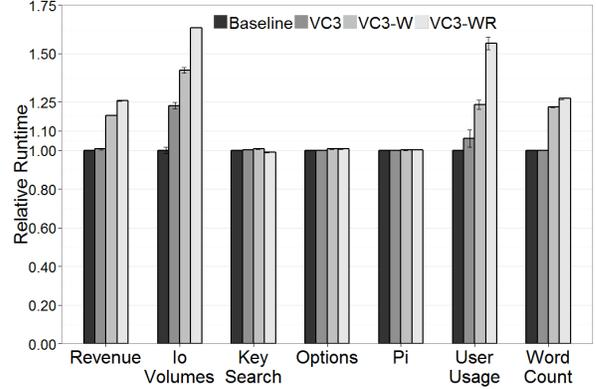
**Fig. 6:** Execution time of running the map phase of MapReduce jobs in isolation over typical input data-sets. Running times are normalized to the performance of running the same computation in the `baseline` configuration.
