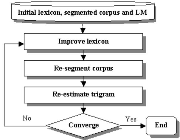
Figure 3. The flowchart of the iterative method for lexicon, segmentation and LM joint optimization
