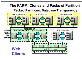
**Figure 5:** A scaled website: showing cloned front ends doing web and firewall service, then shared-disk cloned file servers and packed and partitioned SQL servers.
