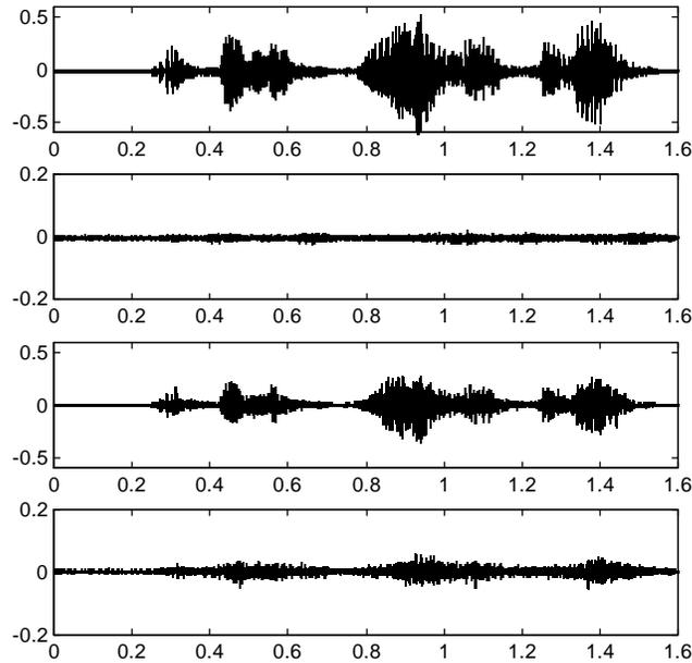
Figure 3. Acoustic echo cancellation experiments. Top: recorded echo return. Second trace: output of a full-band AEC, echo reduction ratio (ERR)  $\approx 26$  dB (note the different vertical scale). Third trace: output of a 512-band MLT AEC without cross filters, ERR  $\approx 5$  dB. Bottom: output of a 512-band MCLT AEC without cross filters, ERR  $\approx 20$  dB.
