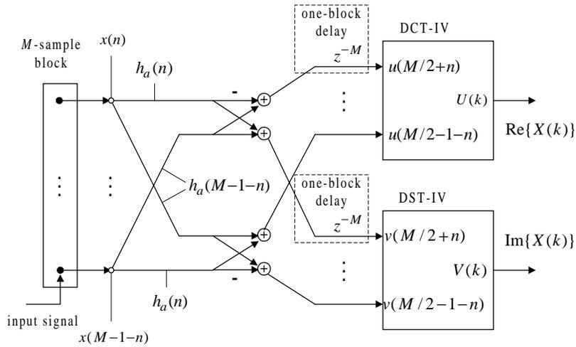
Figure 1. Flowgraph for the fast direct MCLT,  $n = 0, 1, \dots, M/2-1$ ,  $k = 0, 1, \dots, M/2-1$ . The DCT-IV and DST-IV can be implemented with the fast algorithms in [1]. The inverse MCLT can be computed by simply transposing the flowgraph, moving the delays to the bottom half outputs of the DCT-IV and DST-IV [1], replacing the coefficients  $h_a(n)$  by  $h_s(n)$ , and multiplying the contents of the final buffer by  $1/2$ .
