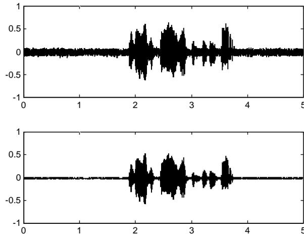
Figure 2. Noise reduction with the CMLT. Top: original speech, corrupted by PC noise, SNR  $\approx$  15 dB. Bottom: processed speech, SNR  $\approx$  30 dB.
