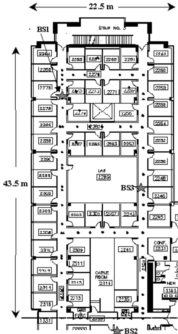
**Figure 1** Map of the floor where the experiments were conducted. The black dots denote locations where empirical signal strength information was collected. The large stars show the location of the three base stations. The orientation is North (up) and East (right).
